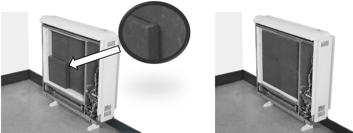
13.- Refit the inner front panel. If the bricks have been fitted correctly you will have no difficulty in refitting the panel. **Make sure the bottom edge of the inner panel is inside the front lip of the heater. Please see below**
