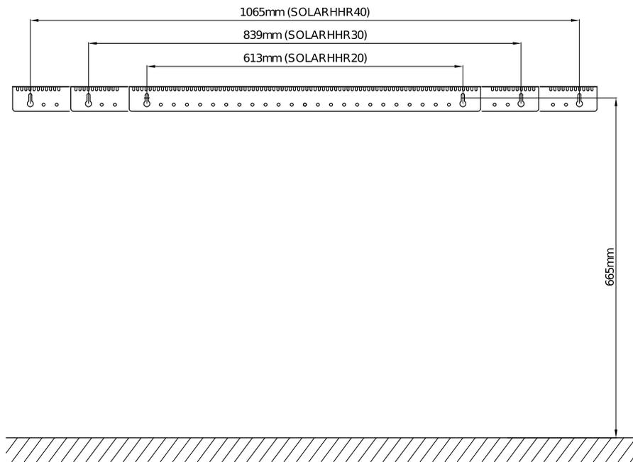
5.- Fix the side fixing plates to the metal casing by using the appropriate screws. The supply cables must be fitted but not wired to the storage heater before placing the heater to the wall. Remove the white screws located in the top of SOLAR HHR, and place the SOLAR HHR in the selected installation area. Use the removed screws to attach SOLAR HHR to the top fixing plate installed in the wall.
