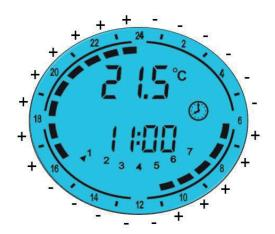
**Note:** In case of loss of power supply, the settings of the "Chrono" mode remain stored in memory for a few minutes.
