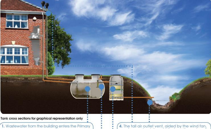
1. Wastewater from the building enters the Primary Tank. Here solids and liquids are separated. The solids are retained and the liquid effluent flows into the FilterPod.
