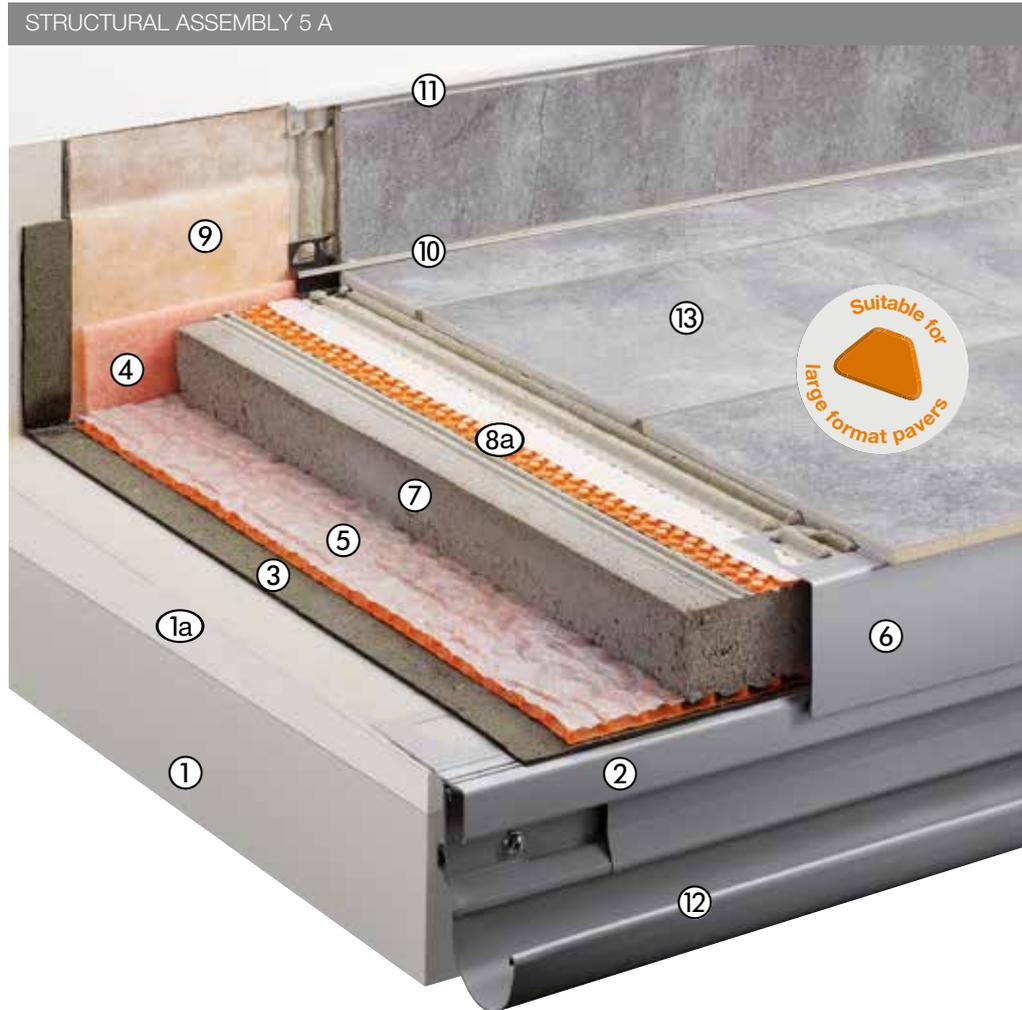
5 A: ASSEMBLY WITHOUT INSULATION, WITH WATERPROOFING
