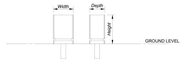
**Dimensions** Width - 605mm, depth - 455mm, height - 890mm. (sizes are approximate)
