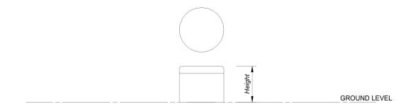
**Dimensions** Available in 400mm diameter, 450mm above ground height. (sizes are approximate)
