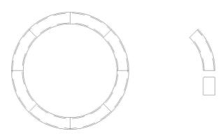
Dimensions Internal diameter 2400mm, External Diameter 3000mm
