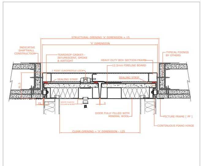
2 hour UL fire rated, picture frame, metal door, 3 point high security lock, double door 4000-2UFR-PF-MD-3HS-DD
