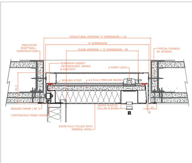
2 hour UL fire rated, beaded frame, metal door, 3 point lock, single door 4000-2UFR-BF-MD-3PL-SD
