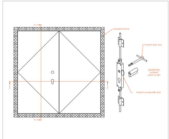
2 hour UL fire rated, beaded frame, metal door, 3 point high security lock, double door 4000-2UFR-BF-MD-3HS-DD
