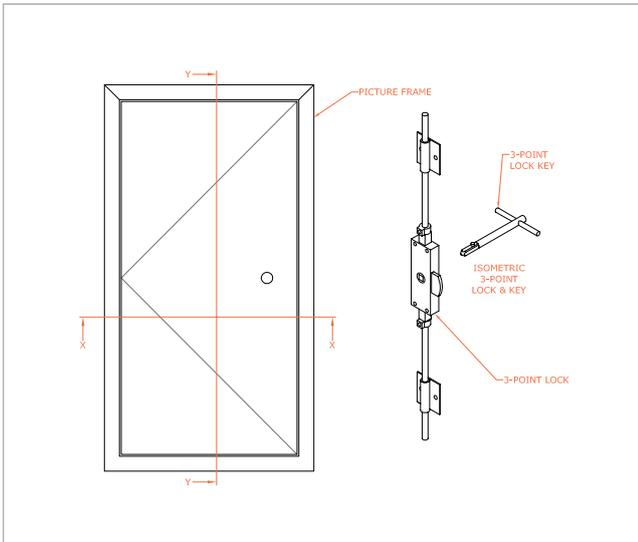
2 hour UL fire rated, picture frame, metal door, 3 point lock, single door 4000-2UFR-PF-MD-3PL-SD
