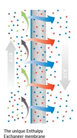
**Summer** - If outside air at 25 deg C and 50% RH passes into a cooled room at 20 deg C the RH would set rise to over 80%. The Enthalpy Exchanger transfers up to 65% of the difference in the moisture levels into the exhaust air preventing this uncomfortable increase from happening.
