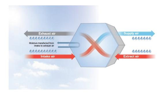
**Winter** - If outside air at 00C and 50% RH is drawn into the home and warmed to 20°C without the addition of any moisture, its RH level would drop to roughly 10%. The Enthalpy Exchanger retains some of the moisture from the extract air and transfers it into the supply air.
