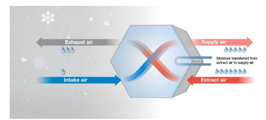
**Comparison** - Compare this to a standard heat exchanger during the winter and it is clear how the indoor climate could become dry and uncomfortable for occupants.
