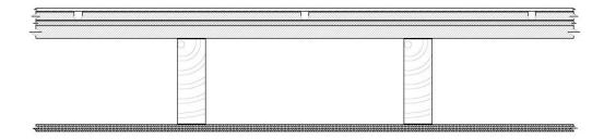
**Airborne sound transmission:** Lowboard RdB improves airborne sound transmission by increasing the amount of sound stopped by the structure from 45dB to 49dB.
