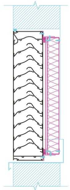
Example: RSH-5700 with an insulated panel - section on elevation
