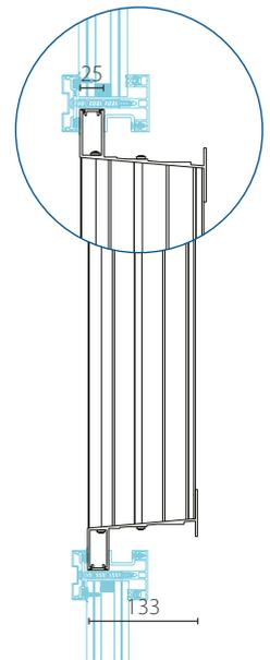
25 mm captured glazing frame with optional snap-on cover plate; spacers can be used to suit wider glazing sockets
