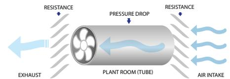
The pressure drop of a louvre will increase with increasing air intake velocities. Too high a pressure drop, and not enough air will be allowed through, causing any HVAC or generator equipment located behind to work harder and overheat.
