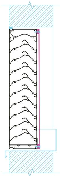
Example: RSH-5700 with a blanking plate - section on elevation
