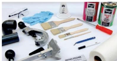
The additional range of preparation tools and installation equipment ensures a safe, efficient and simple jointing process. Time saving "dry fit" installations on PVC-U are most of the time possible due to our excellence in production and tight tolerances.
