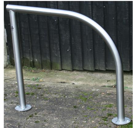
The Kingsthorpe Cycle Stand is a shaped tubular cycle stand. The design allows the frame of the bicycle to be secured by the users own security lock. The Kingsthorpe Cycle Stand is suitable for securing two bicycles. The Kingsthorpe Cycle Stand is available in galvanised steel or grade 304 stainless steel, with ragged feet for casting into new concrete or flanged feet for bolting to an existing surface.
