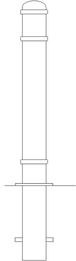
The GFC1900 (Slough) Ornamental Mild Steel Bollard from AUTOPA is suitable for a wide range of locations and purposes. Constructed using mild steel, then galvanised to ensure its longevity. Cap and rings are welded onto the steel tube to complete the design.
