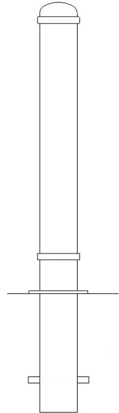
The GFC1200 (Delaval) Ornamental Mild Steel Bollard from AUTOPA is suitable for a wide range of locations and purposes. Constructed using mild steel, then galvanised to ensure its longevity. Cap and rings are welded onto the steel tube to complete the design.
