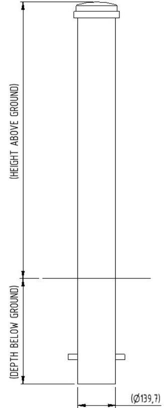
The GFC9000 Ornamental Mild Steel Bollard from AUTOPA is suitable for a wide range of locations and purposes. Constructed using mild steel, then galvanised to ensure its longevity. Cap is welded onto the steel tube to complete the design.
