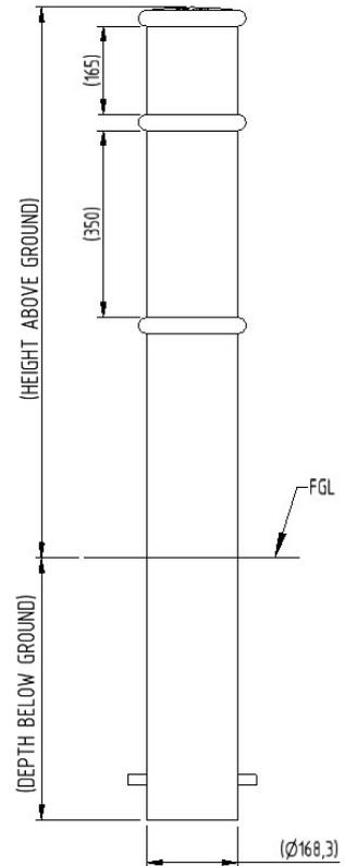
The GFC6000 Ornamental Mild Steel Bollard from AUTOPA is suitable for a wide range of locations and purposes. Constructed using mild steel, then galvanised to ensure its longevity. Cap and rings are welded onto the steel tube to complete the design.
