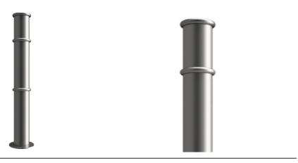
The GFC3000 Ornamental Mild Steel Bollard from AUTOPA is suitable for a wide range of locations and purposes. Constructed using mild steel, then galvanised to ensure its longevity. Cap and rings are welded onto the steel tube to complete the design.
