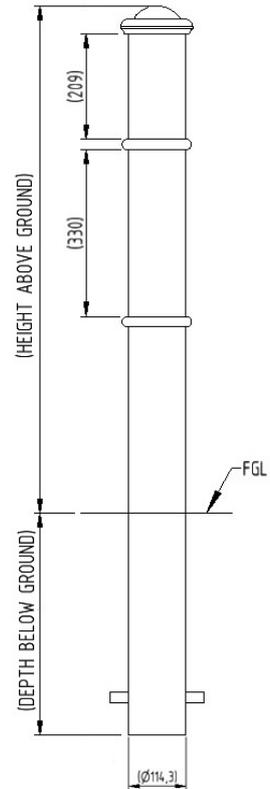
The GFC1500 Ornamental Mild Steel Bollard from AUTOPA is suitable for a wide range of locations and purposes. Constructed using mild steel, then galvanised to ensure its longevity. Cap and rings are welded onto the steel tube to complete the design.
