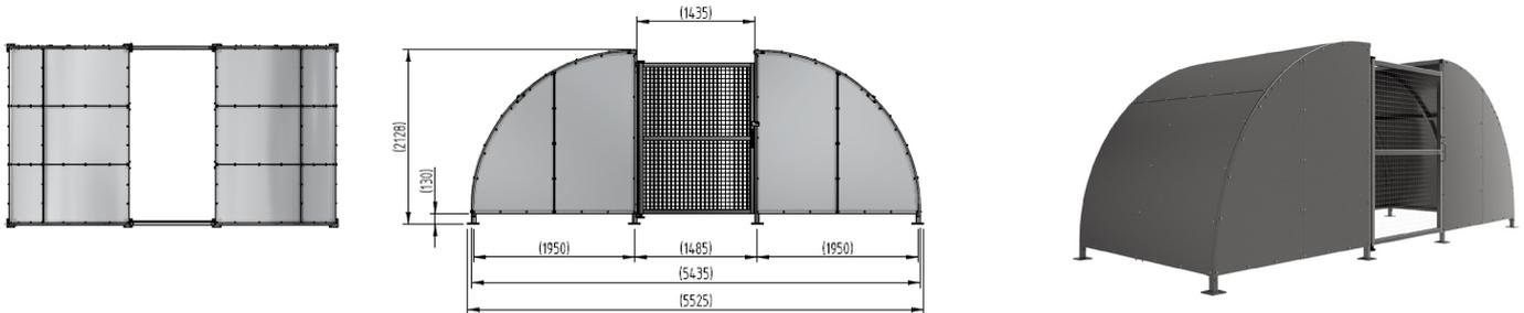
The Stratford Compound is a free-standing shelter with a Mesh Door lockable by padlock (not included) designed for on site assembly, constructed from galvanised mild steel. Complete with a galvanised sheet curved roof and end panels.
