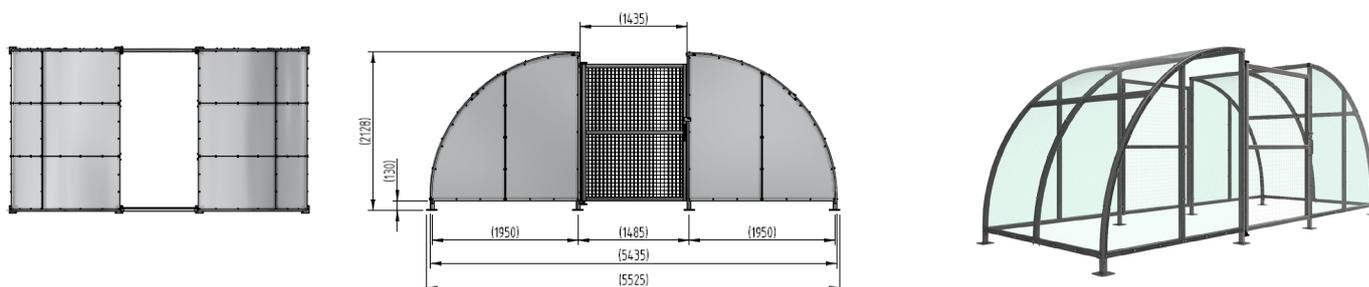
The Stratford Compound is a free-standing shelter with a Mesh Door lockable by padlock (not included) designed for on site assembly, constructed from galvanised mild steel. Complete with a 4mm PETG clear sheet curved roof and end panels.
