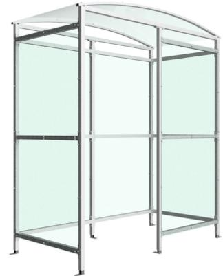
The Formby shelter is a free-standing, open sided shelter designed for on site assembly, constructed from aluminium. Complete with a 4mm PETG clear sheet roof, and side panels. Front-to-back curved roof. Coated RAL7016 (anthracite grey) as standard, other standard RALs available on request.
