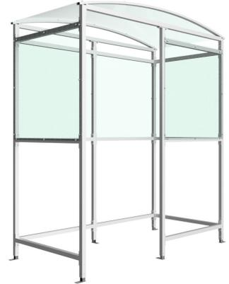
The Cannock shelter is a free-standing, open fronted shelter designed for on site assembly, constructed from aluminium. Complete with a 4mm PETG clear sheet roof, and ½ side panels. Side-to-side curved roof. Coated RAL7016 (anthracite grey) as standard, other standard RALs available on request.
