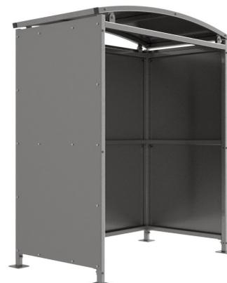
The Binley shelter is a free-standing, open fronted shelter designed for on site assembly, constructed from galvanised mild steel. Complete with galvanised sheet roof, and side panels. Side-to side curved roof.
