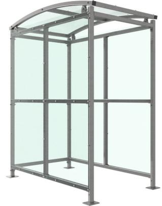
The Badby shelter is a free-standing, open sided shelter designed for on site assembly, constructed from galvanised mild steel. Complete with a 4mm PETG clear sheet roof, and side panels. Front-to-back curved roof.
