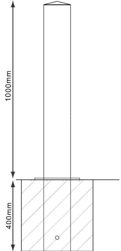
The AUTOPA Diamond Top Bollard is a square, galvanised mild steel bollard with a pressed steel, fully welded cap. The Diamond Top Bollard is an elegantly simple bollard, ideal for providing protection against unauthorised parking or access. The Diamond Top Bollard is ideal for use around pedestrian precincts, pavements, play and parking areas, as part of traffic calming measures, pedestrianisation schemes and as a deterrent to ram-raiders.
