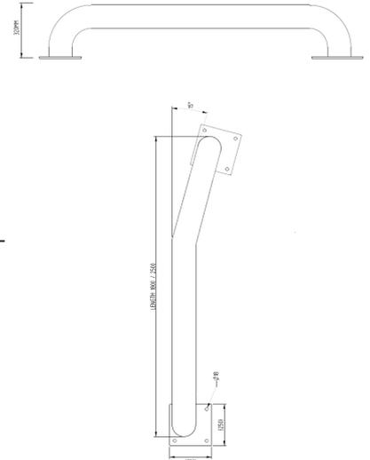
The AUTOPA Cranked HGV wheel guides provide a solid, steel kerb to allow the safe reversing into loading bays by wagons and delivery trucks. Also suitable for protecting racking, equipment and machines from potential damage caused by forklift trucks and moving vehicles.
