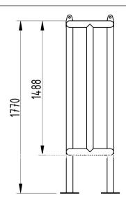
Functional and robust in design, AUTOPA's range of vertical column protectors are designed to protect pipes and other vulnerable pillars from vehicle damage in a busy industrial environment. Manufactured from mild steel and galvanised to ensure their longevity. Suitable for both internal and external use.
