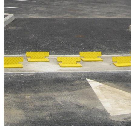
The AUTOPA One Way Flow Plate controls traffic flow to one direction only and is designed to work in groups to provide full road width coverage. As a vehicle passes over the plate, the flap is pushed down, allowing the vehicle to pass, the rubber buffer on the reverse of the flap ensures noise is kept to a minimum. Once the vehicle has passed the flap returns to its upright position.
