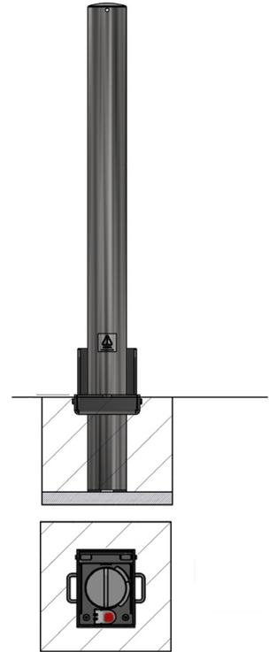
The RGP (removable ground post) offers a highly effective and robust way to protect premises and vehicles. The post is 900mm above ground, when removed the socket is covered using the integral lid. The post is lockable by rotating the post 45° and then pressing the high-security push button 7-pin security lock. The post is unlocked using the supplied key, rotated and then removed.
