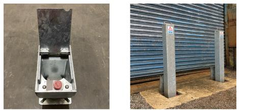
The RGP (removable ground post) offers a highly effective and robust way to protect premises and vehicles. The post is 900mm above ground, when removed the socket is covered using the integral lid. The post is lockable by rotating the post 45° and then pressing the high-security push button 7-pin security lock. The post is unlocked using the supplied key, rotated and then removed.
