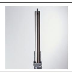
The RGP (removable ground post) offers a highly effective and robust way to protect premises and vehicles. The post is 745mm above ground, when removed the socket is covered using the integral lid. The post is lockable by rotating the post 45° and then pressing the high-security push button 7-pin security lock. The post is unlocked using the supplied key, rotated and then removed.
