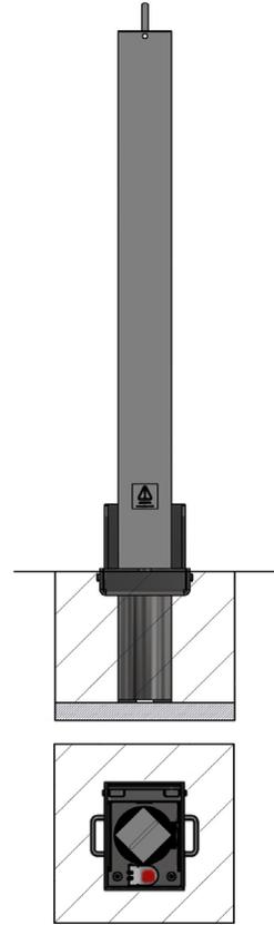
The RGP (removable ground post) offers a highly effective and robust way to protect premises and vehicles. The post is 745mm above ground, when removed the socket is covered using the integral lid. The post is lockable by rotating the post 45° and then pressing the high-security push button 7-pin security lock. The post is unlocked using the supplied key, rotated and then removed.
