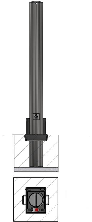
The RGP (removable ground post) offers a highly effective and robust way to protect premises and vehicles. The post is 500mm above ground, when removed the socket is covered using the integral lid. The post is lockable by rotating the post 45° and then pressing the high-security push button 7-pin security lock. The post is unlocked using the supplied key, rotated and then removed.
