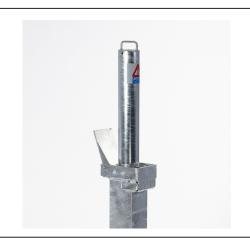
The RetractaPost-GL offers a highly effective and robust way to protect premises and vehicles. The RetractaPost-GL is raised and lowered vertically. When raised the post is 500mm above ground, when lowered the post is fully below ground and covered using the integral lid. The post is lockable in the raised position by rotating the post 45° and then pressing the high-security push button 7-pin security lock. The post is unlocked using the supplied key, rotated and then lowered.
