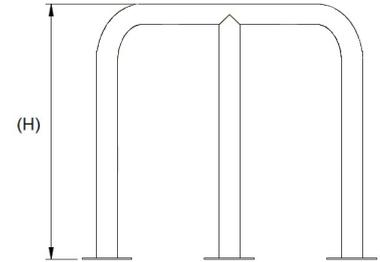
The AUTOPA Corner Protection Hoop provides protection for corners and other vulnerable areas on busy industrial sites. Manufactured from mild steel and galvanised for longevity, the Corner Protection Hoop is highly durable. Available in 500mm and 800mm heights they can be used to protect a wide range of locations from vehicles of different sizes.
