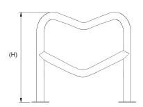
The AUTOPA Corner Protection Hoop provides protection for corners and other vulnerable areas on busy industrial sites. Manufactured from mild steel and galvanised for longevity, the Corner Protection Hoop is highly durable. Available in 500mm and 800mm heights they can be used to protect a wide range of locations from vehicles of different sizes.
