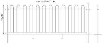
AUTOPA's Bow Top Fencing Rail is ideal for residential and commercial properties to mark and secure site perimeters. All the products in the range are manufactured by AUTOPA from mild steel which is galvanised for longevity. The fence panels are supplied galvanised as standard and can be colour coated if required. RAL numbers must be specified at time of
