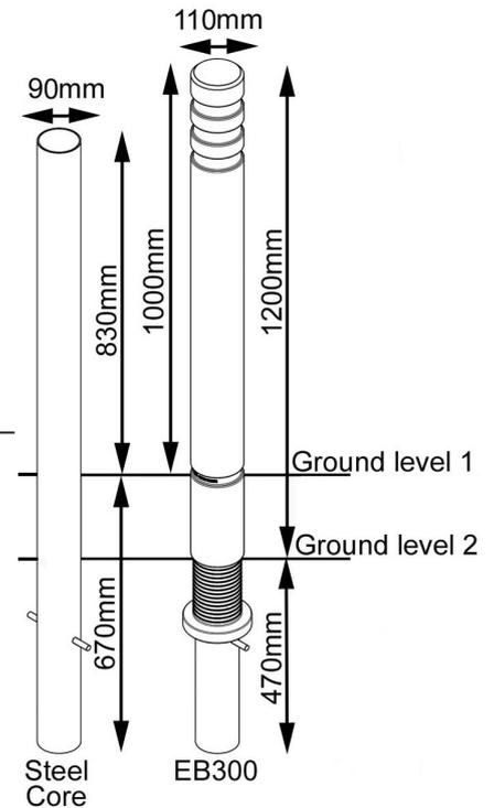
With a unique, slimline design, the EB300 bollard from AUTOPA is ideal for marking paths where space is at a premium. The EB300 bollard is highly versatile and features a galvanised steel core covered by a hard wearing medium density polyethylene (MDPE) sleeve. When complete with the core, this bollard can be installed at either 1000mm or 1200mm height above ground.
