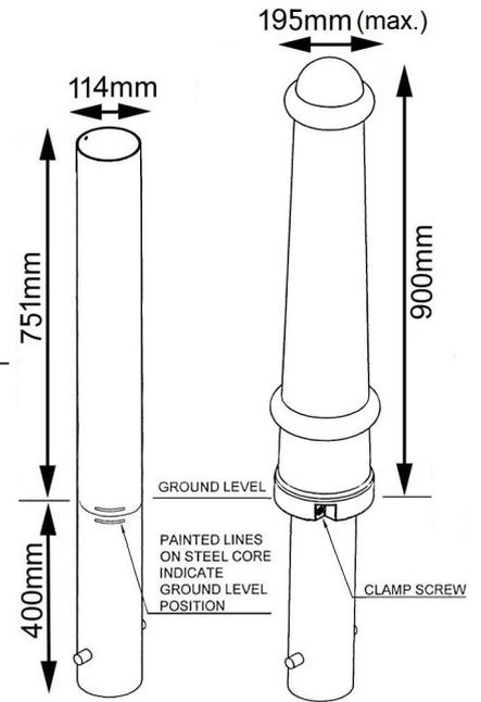
With a traditional design, the EB200 offer a durable alternative to a cast iron bollard. Highly versatile and suited for a wide range of applications, the AUTOPA EB200 houses a galvanised steel core under a rugged medium density polyethylene (MDPE) sleeve. The combination of steel and MDPE make the EB200 100% recyclable. The sleeve is fully removable, and can be easily replaced if damaged.
