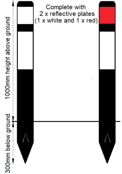
The Fleximarker Verge Marker is highly durable and suited to a wide range of roadside locations. Manufactured from UV resistant plastic, this verge marker complies with BS EN 1276-7. The Fleximarker flexes up to 90 degrees, returning to its upright position, and will not splinter in the event of an impact.
