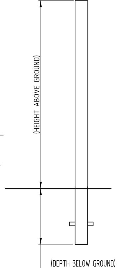
The galvanised mild steel range of 900mm tall square fixed bollards are suitable for a range of applications and are ideal as a complement to the Autopa ranges of square Parking Posts, RemovaPosts and RetractaPosts.
