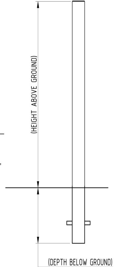
The galvanised mild steel range of 900mm tall square fixed bollards are suitable for a range of applications and are ideal as a complement to the Autopa ranges of square Parking Posts, RemovaPosts and RetractaPosts.
