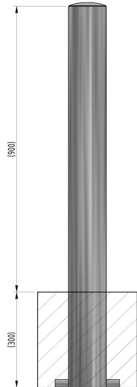
The galvanised mild steel range of 900mm tall fixed bollards are suitable for a range of applications and are ideal as a complement to the Autopa ranges of Parking Posts, RemovaPosts and RetractaPosts.
