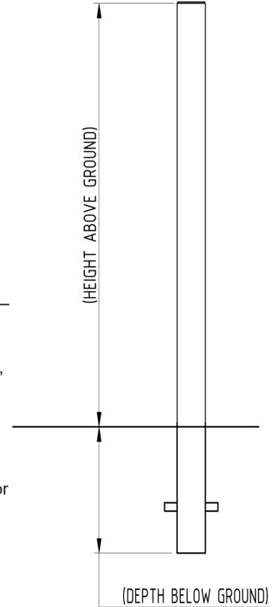
The galvanised mild steel range of 750mm tall square fixed bollards are suitable for a range of applications and are ideal as a complement to the Autopa ranges of square Parking Posts, RemovaPosts and RetractaPosts.
