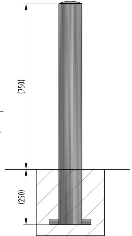
The stainless steel range of 750mm tall fixed bollards are suitable for a range of applications.
