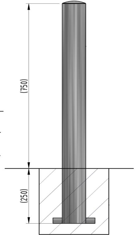
The stainless steel range of 750mm tall fixed bollards are suitable for a range of applications.
