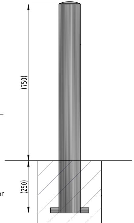
The galvanised mild steel range of 750mm tall fixed bollards are suitable for a range of applications and are ideal as a complement to the Autopa ranges of Parking Posts, RemovaPosts and RetractaPosts.
