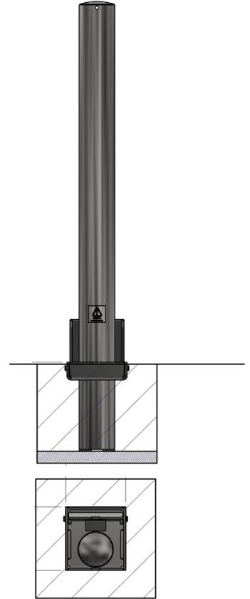
The Removable Bollard offers an effective, simple and robust way to protect premises and vehicles. Removable Bollards are particularly suitable for locations where occasional access is required, the simple tab and padlock system provides an easy to operate solution for locking the bollard in place. The Removable Bollard is 1,000mm above ground and is available in a range of outside tube diameter sizes from 60mm through to 219mm. Padlock to secure is available at an extra cost.
