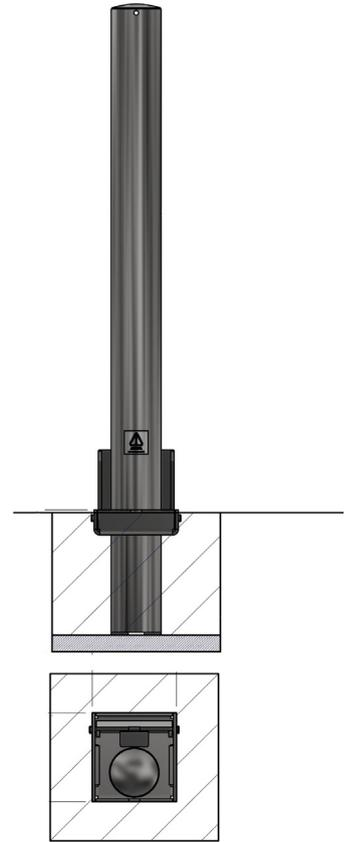
The Removable Bollard offers an effective, simple and robust way to protect premises and vehicles. Removable Bollards are particularly suitable for locations where occasional access is required, the simple tab and padlock system provides an easy to operate solution for locking the bollard in place. The Removable Bollard is 900mm above ground and is available in a range of outside tube diameter sizes from 90mm through to 168mm. Padlock to secure is available at an extra cost.
