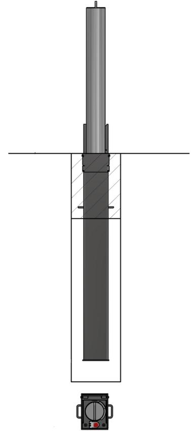
The RetractaPost-GL offers a highly effective and robust way to protect premises and vehicles. The RetractaPost-GL is raised and lowered vertically and is 900mm tall when raised. When lowered the post is fully below ground and covered using the integral lid. The post is lockable in the raised position by rotating the post 45° and then pressing the high-security push button 7-pin security lock. The post is unlocked using the supplied key, rotated and then lowered.
